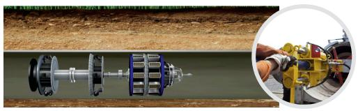
• Pipeline operators inspect their lines using devices called "smart pigs" to monitor pipelines from within. Smart pigs have on-board diagnostic systems, which can identify problems in the pipe wall due to corrosion, cracking or other sources of damage.
